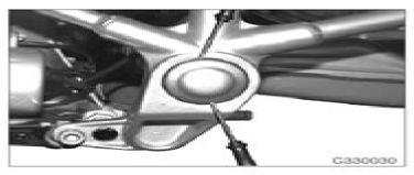
Press off left swinging arm bearing cap.
