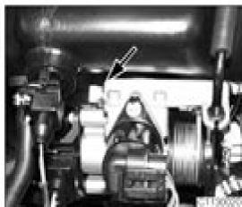
Loosen plenum chamber/throttle valve hose clamp (arrow)
