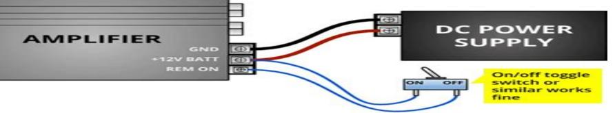
Example 3 If you're using a line level converter, you can optionally use one with a remote wire output built in. The amp will turn on and off automatically with the speaker level input signal. These types need power to be connected also.
