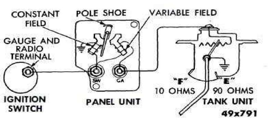
Fig. 12 - Electro-Magnetic Fuel Gauge Circuit
