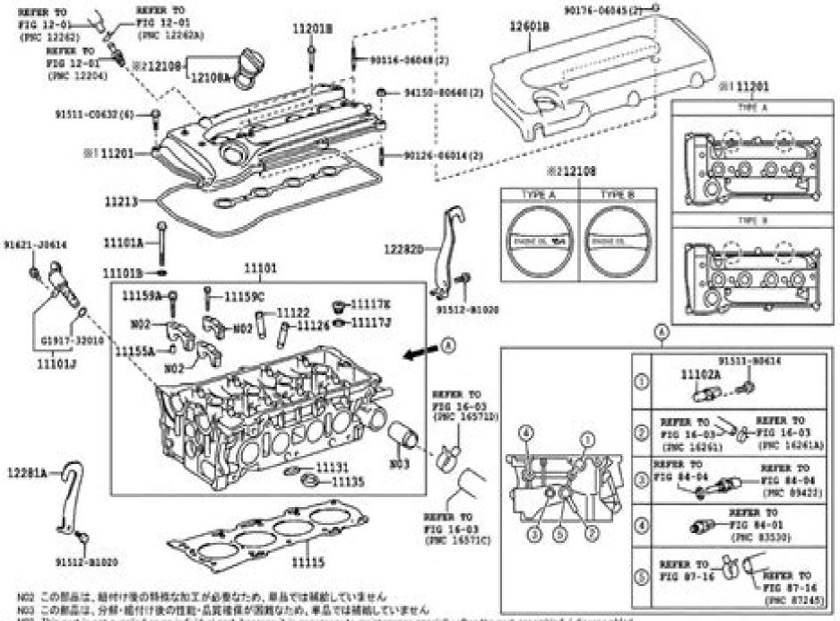
P NOS. This part is not supplied as an individual part, because it is necessary to maintenance openially after the part assembled / disassembled. NOS. This part is not supplied as an individual part, because it is difficult to keep the function / quality of parts, assembled / disassembled.
