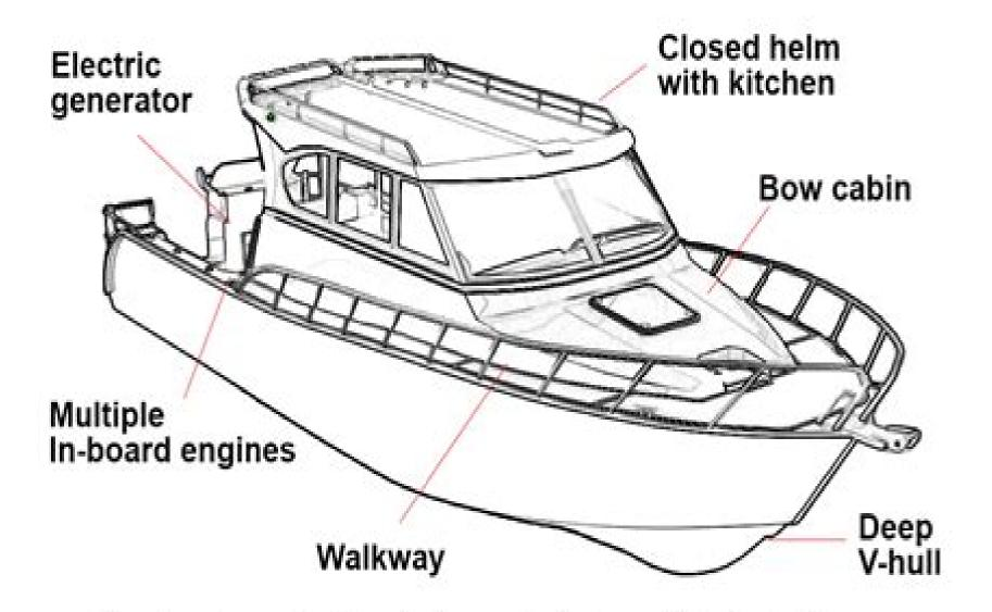
The cabin cruiser provides the optimal compromise between a fishing boat and luxury cruiser—without the sticker shock. Ideal for longer fishing trips, where comfort is a must. The deep-V design and inboard motor ensures solid performance. (source:norrik.com)
