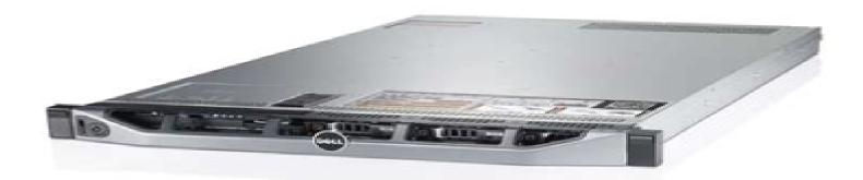
This hyper-dense, two-socket, 1U rack server has a large memory footprint and impressive I/O options that make it exceptional for space-sensitive environments.
