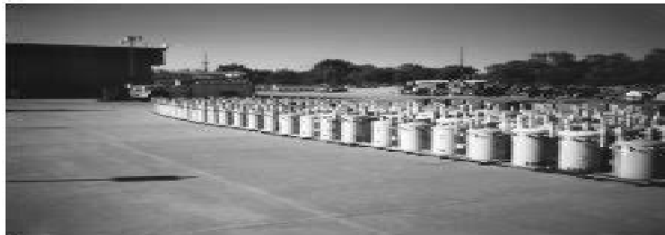
FIGURE 15.1 Electric utility distribution storage yard. Forklift trucks are used to load transformers on line trucks. Storage area is covered with concrete to provide accessibility and protect transformers.
