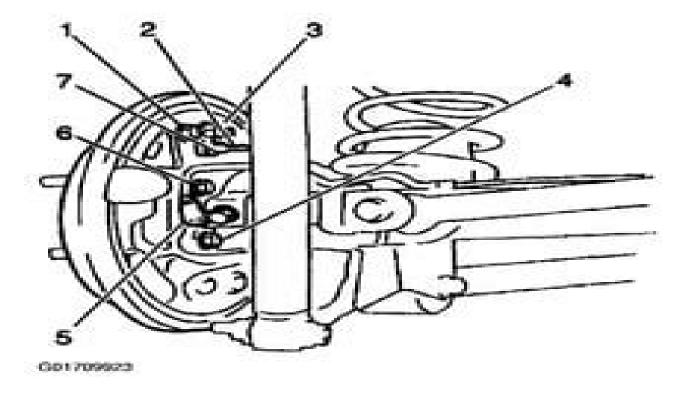
Fig. 13: Removing Nuts From Bearing Retainer Studs Courtesy of GENERAL MOTORS CORP.
