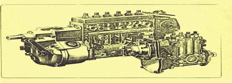
Fuel Injection Equipment for Diesel Engines Governors for In-Line Pumps
