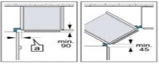
To ensure that the appliance door can be opened, you must take the minimum dimensions into consideration when installing in a corner. The dimension (a) is dependent on the thickness of the unit front and the handle.
