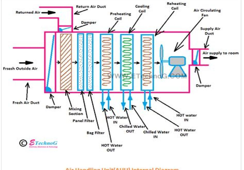
Air Handling Unit(AHU) Internal Diagram
