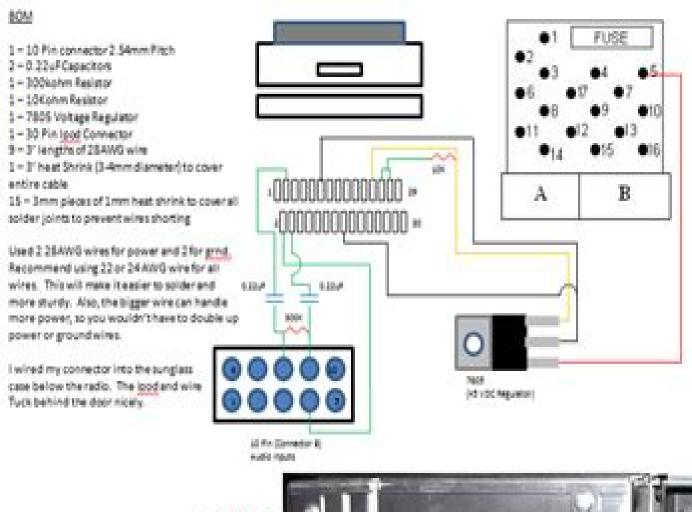
Pin 2 - Audio Gred Pin 3 - Line Out Right Pin 4 - Line Out Left Pin 11 - Activates Line Out Audio
