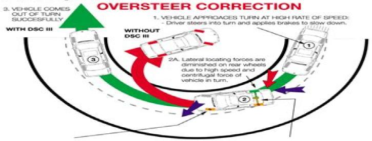
2D. The torque reduction and rear brake regulation should stabilize the vehicle at this point, if not the left front wheel has a high degree of lateral locating force and is momentarily regulated.
