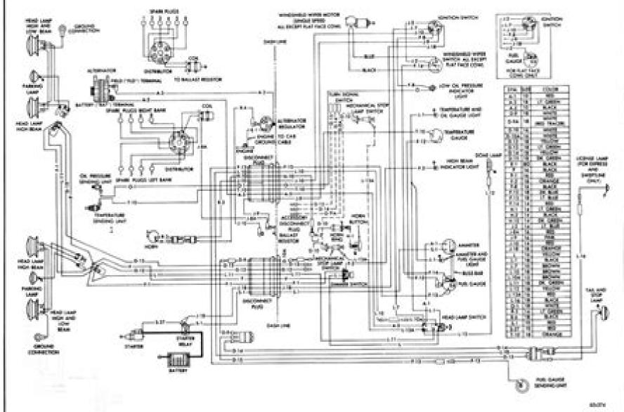
Fig. 10—Wiring Diagram (Cab, Cawl, Platform and Stake) D100-0600, D100-W500
