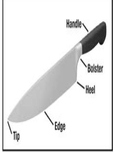
Figure 1. Model 120 EdgeSelect Diamond Hone® Sharpener. Figure 2. Typical kitchen knife.
