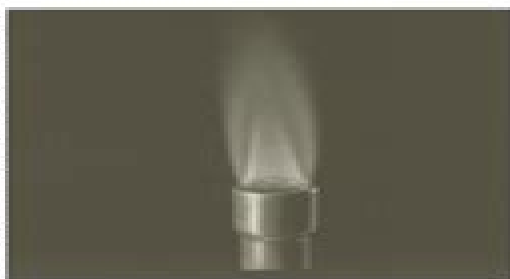
A properly adjusted Bunsen flame is a blue, nonluminous flame.
