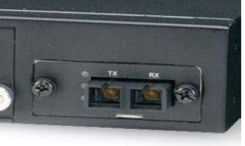
The half-slot LBB220C-ST-R2 module adds one fiber ST uplink to the LB9217A-R2.
