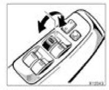
Automatic operation: Push the switch completely down or pull it completely up, and then release it. The window will fully open or close. To stop the window partway, lightly move the switch in the opposite direction and then release it.
