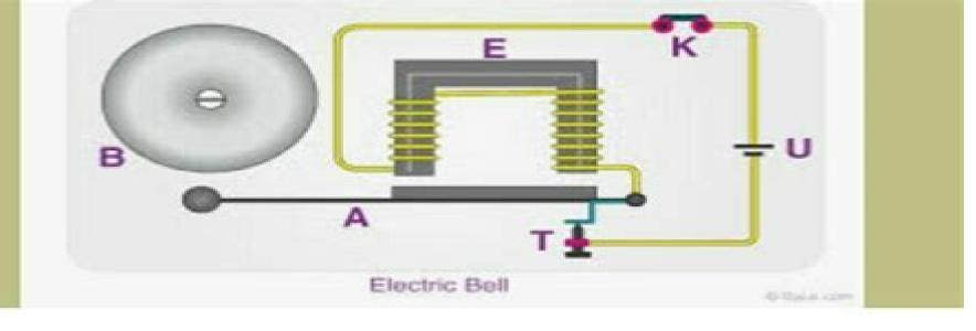
Process of the working of an electric bell
