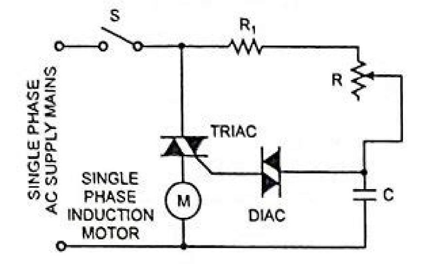
Fig. 3.55. Speed Control of Single Phase Induction Motor using Triac (Fan Regulator)
