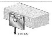
1.45 Three 18-mm-diameter steel bolts are to be used to attach the steel plate shown to a wooden beam. Knowing that the plate will support a 110-kN load and that the ultimate shearing stees for the steel used is 360 MPa, determine the factor of safety for this design.
