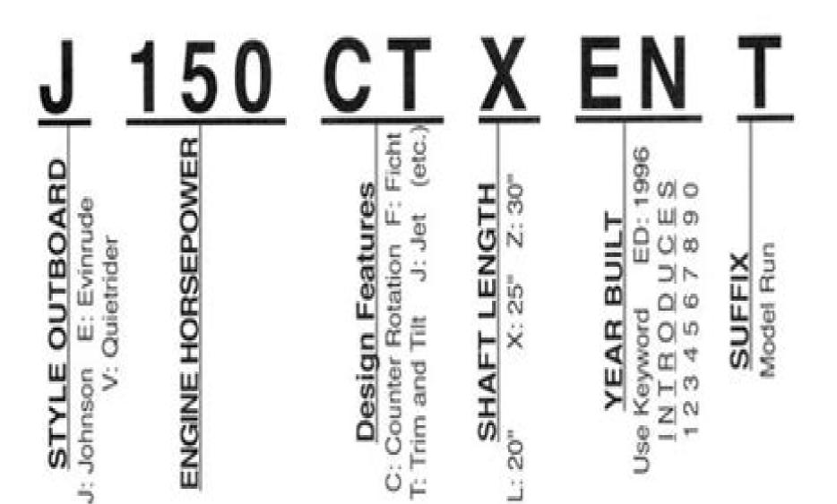
The example above represents a Johnson, 150HP, counter rotating, with tilt and trim system. 25" Iona drive shaft. 1992 year model.
