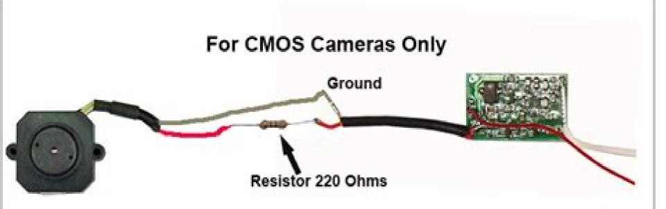
Note: For CMOS Cameras, Add Serial Resistor 220 Ohms to Video Input
