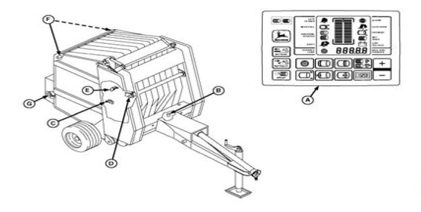
A-Monitor-Controller (located C-Gate Close Switch on tractor). B-Twine Wrap Sensor
