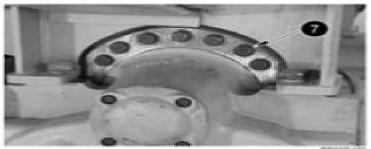
Remove the seven bolts (7) and washers (8) securing the final drive to the transmission housing.
