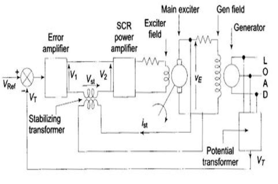
Fig. 8.20 Schematic diagram of alternator voltage regulator scheme
