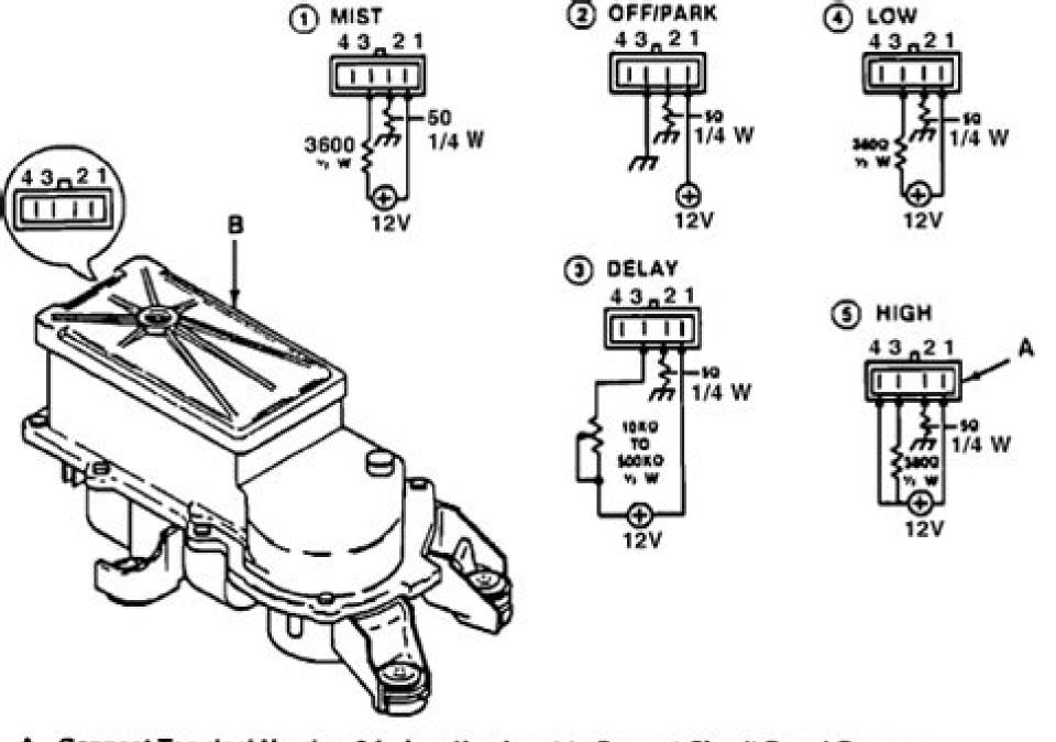
A. Connect Terminal Number 3 before Number 4 to Prevent Circuit Board Damage B. Maximum Operating current 5.0 Amperes
