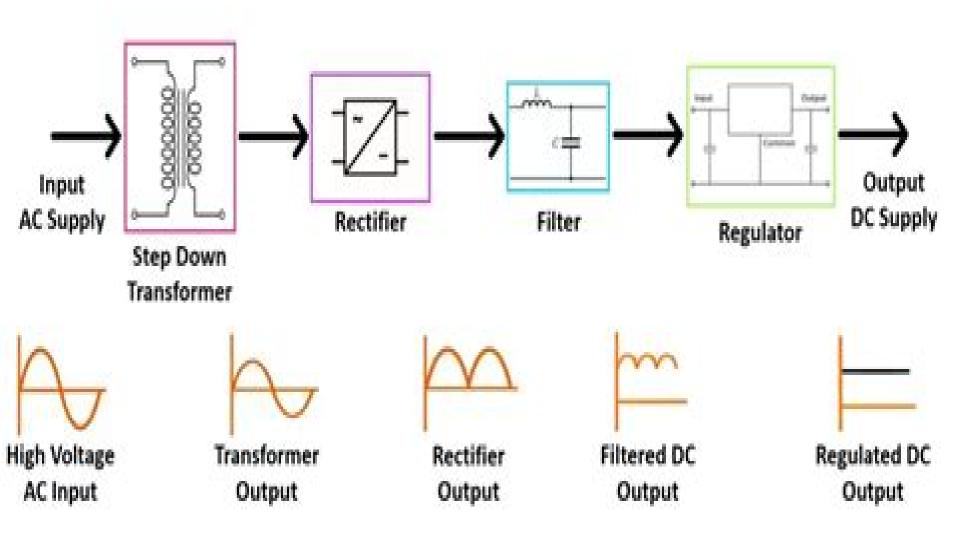
Linear Regulated Power Supply Block Diagram
