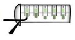
7 Once you set the final pin, the plug will be free to rotate, just as if the proper key had been inserted.
