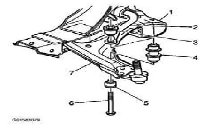
Fig. 6: Stabilizer Link Courtesy of GENERAL MOTORS CORP.
