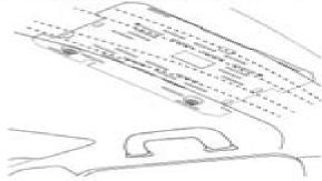
Choose suitable size of screw to install the stand. Before tightening the screw on the stand, pull the wire rod of the wire hole out.
