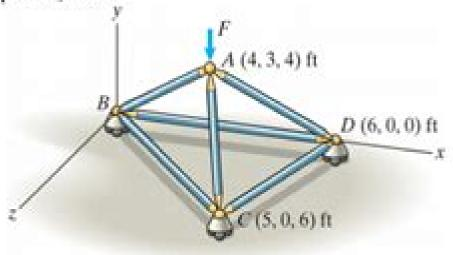
Statics analysis has been performed and the following equations are obtained relating the applied force and the axial forces in members AB, AC, and AD, which are most likely to fail compared to other members:
