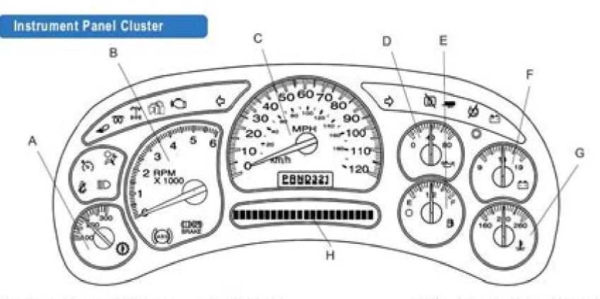
Your vehicle's instrument panel is equipped with this cluster or one very similar to it. The U.S. Heavy-Duty Automatic Transmission version is shown here.
