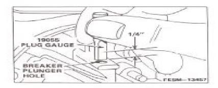
If the flat end of the 19055 plug gauge will enter the plunger hole a distance of 6.4 mm (1/4 inch) or more, the hole is worn excessively.
