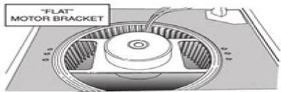
Determine which MOTOR BRACKET is used in your fan.
