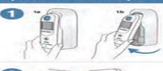
Remove thermometer from cradle by gripping thermometer at base and pivoting up.
