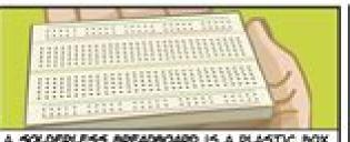
A SOLDERLESS BREADBOARD IS A PLASTIC BOX FULL OF METAL STRIPS, WITH A GRID OF HOLES ON TOP. IT IS USED TO BUILD AND TEST CIRCUIT'S QUICKLY.
