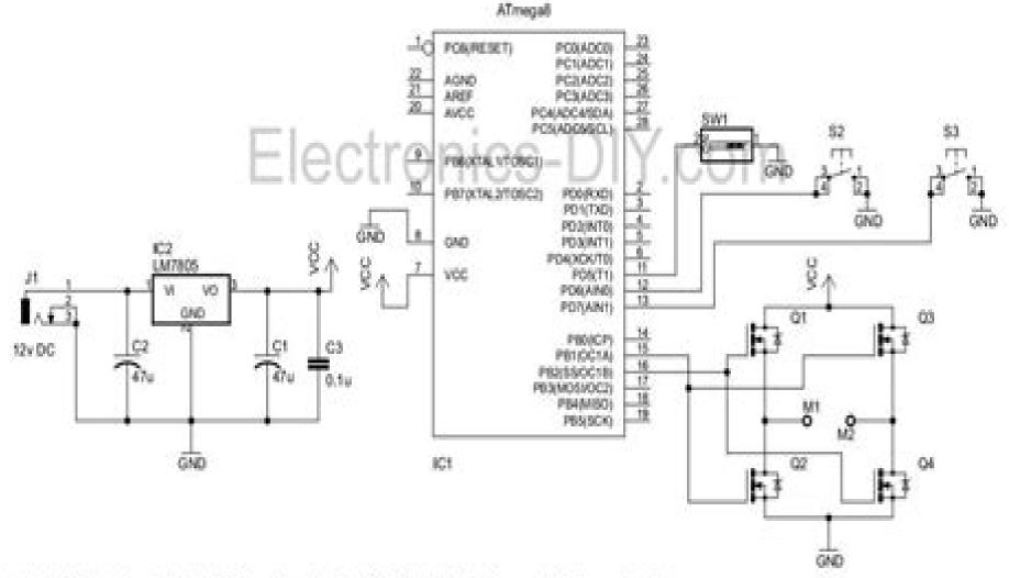
Small DC Motor Control by PWM method using MOSFET H-Bridge with ATmega8 uC
