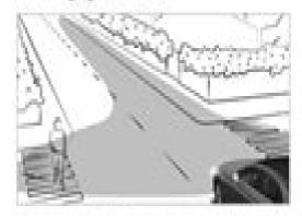
The cornering light improves the illumination of the road over a wide angle in the turning direction, enabling better visibility on tight curves, for example, it can be activated only when the low beam is switched on.
