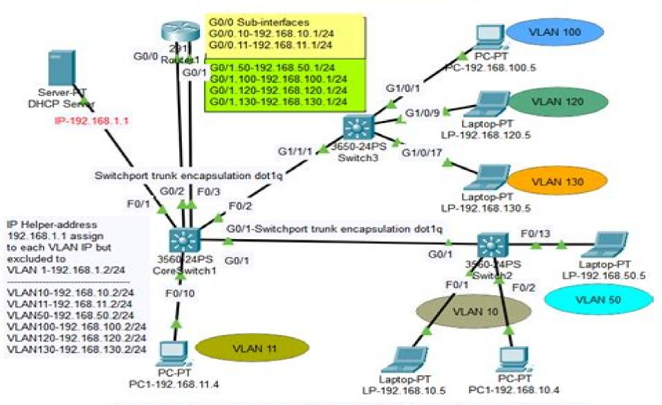
VLAN clients obtaiend ip address from DHCP Server after configuration of IP Helper-address.
