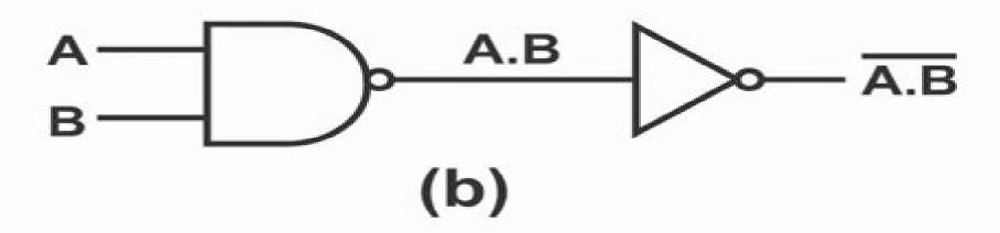
Fig 2.24 (a) NAND gate logic symbol. (b) A Boolean expression for the output of a NAND gate
