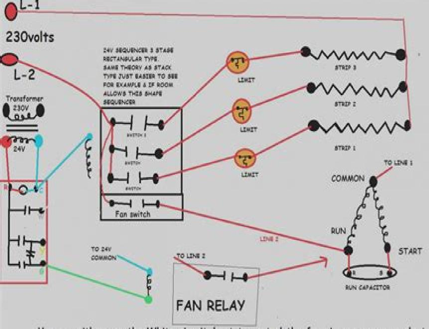
You can either use the White circuit=heat, to control the fan via sequencer or electric heat thermostat to control the fan in both heat and cool modes.
