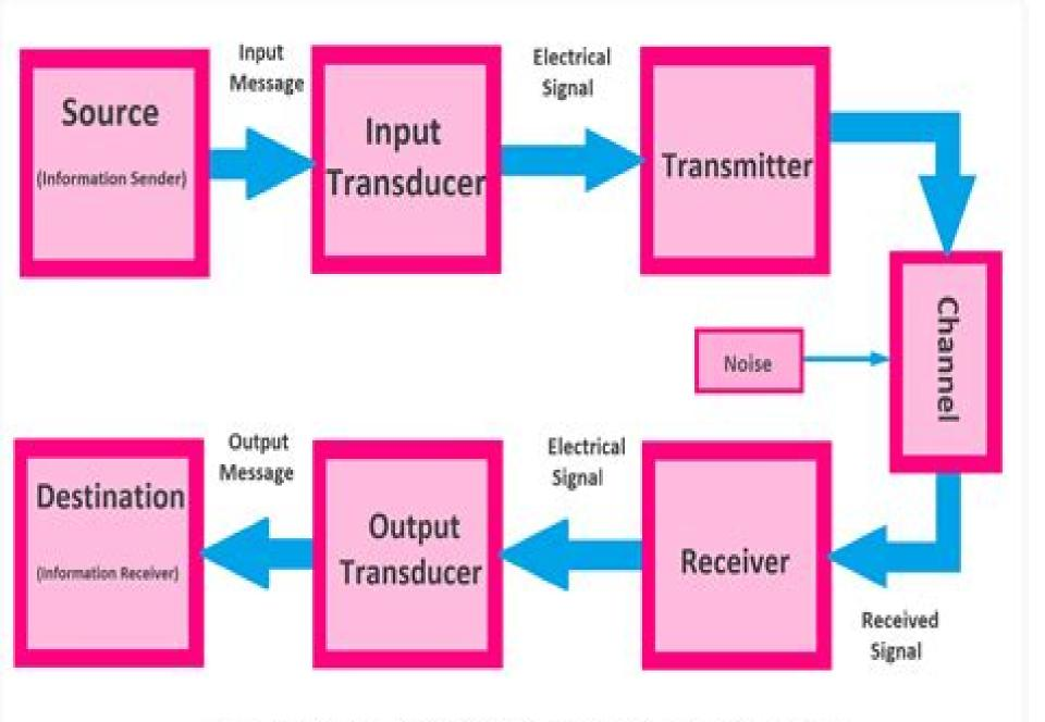
Basic Communication System Block Diagram
