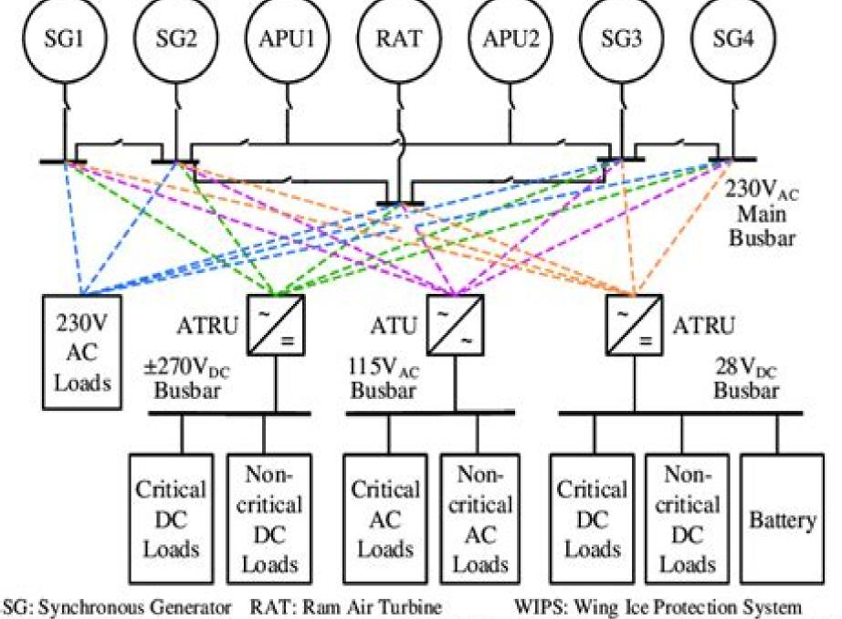
APU: Auxiliary Power Unit ATU: Auto Transformer Unit ATRU: Auto Transformer Rectifier Unit
