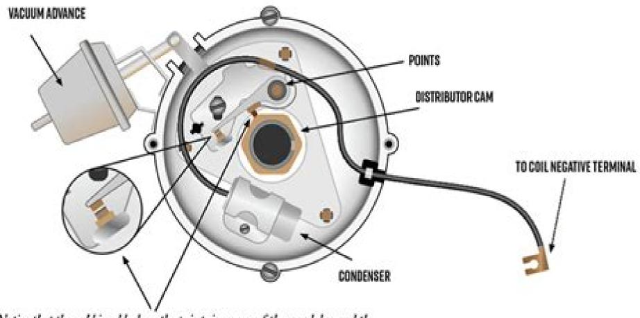
Notice that the rubbing block on the points is on one of the cam lobes and the contacts are open. Current flow through the coil is interrupted, creating high voltage in the secondary side of the ignition coil.
