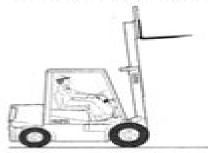
If the maximum fork height cannot be reached, this indicates there is low oil level in the hydraulic sumpor severe binding within the upright.
