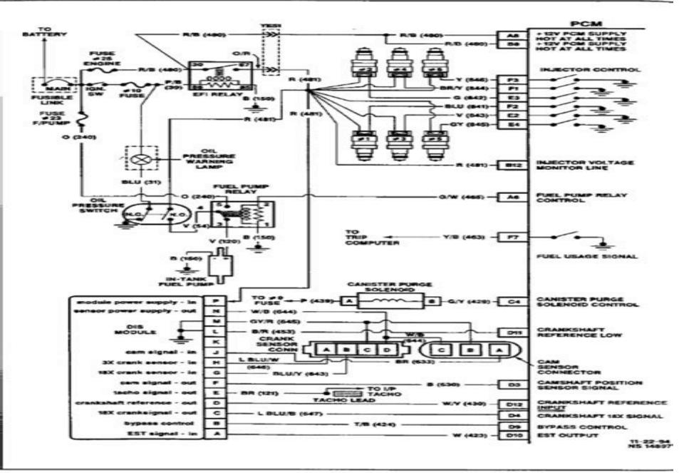
Figure 6C1-2A-5 V6 PCM Wiring Diagram (1 of 5)
