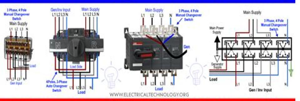
Three Phase Auto & Manual Changeover / Transfer Switch Connection & Wiring
