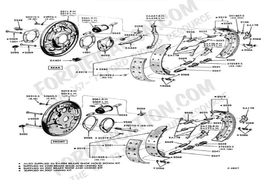
FRONT & REAR BRAKES - SELF ADJUSTING - TYPICAL 1964/72 E100/200, F100 (4 x 2) P100 1967 F100 (4 x 4), F250, P350/400
